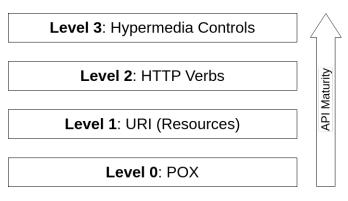
Figure 3.3: The four levels to reach REST [15][41]
