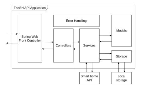
Figure 6.5: High level API application architecture
