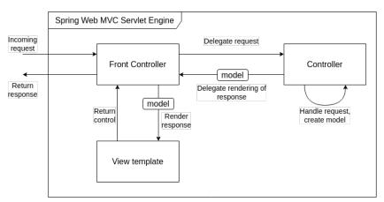
Figure 6.2: Spring Web MVC Servlet Engine [49]
