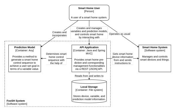
Figure 6.4: C4 Level 2 - Container Diagram
