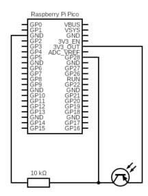
Figure 7.2: Measurement Station Circuit Schematic
