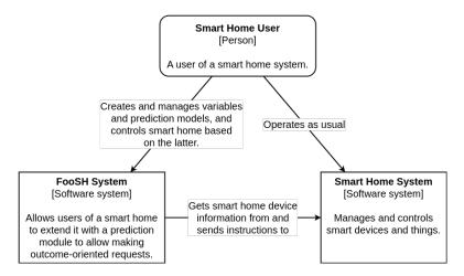
Figure 6.1: C4 Level 1 - Architecture Context Diagram
